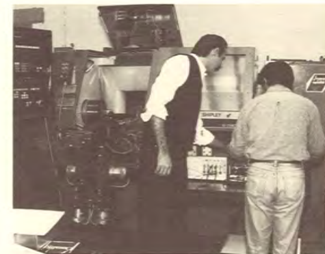
Prof. Galip Ulsoy's real time tool-wear instrumentation is evaluated on a turret lathe in the MEAM machine tool laboratory. The method uses force measurements during cutting, together with a process model.
