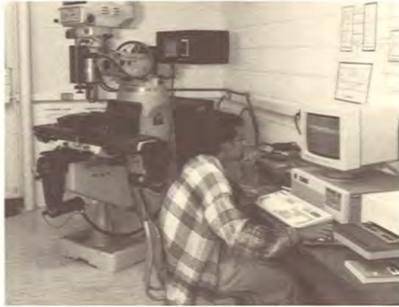
Cross coupling control developed by Prof. Yoram Koren allows this milling machine to produce more accurate contour machining.
