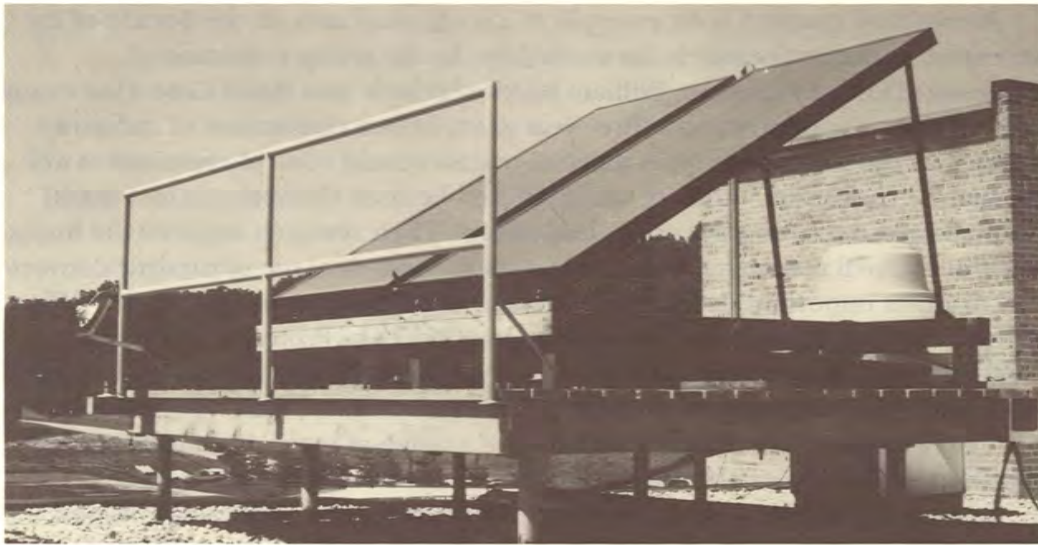
Professor John Clark's investigation of solar energy is an example of an ongoing commitment to new fields of scientific inquiry that characterizes research in the Department of Mechanical Engineering and Applied Mechanics. Pictured here is one of two large solar arrays used in Clark's research that were mounted on the roof of the G.G. Brown Building. These panels absorbed heat directly and used a circulating liquid as a transport medium.
