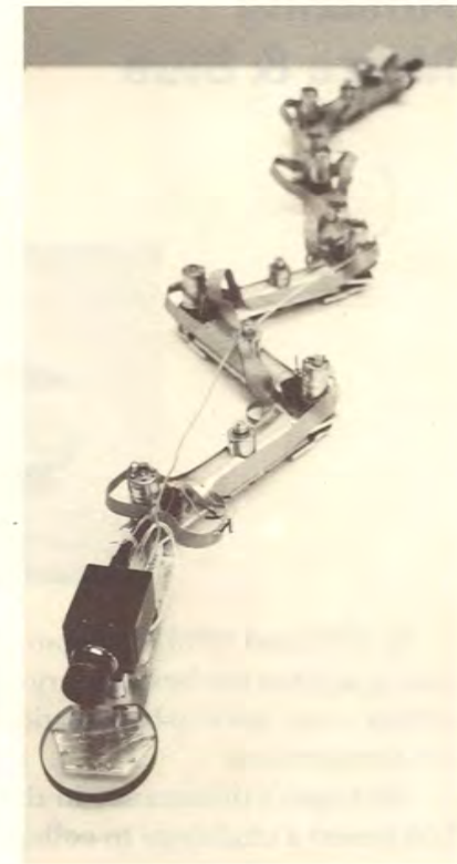
The mechanical snake robot is designed to operate in settings that are too hazardous or too constricted for humans to enter.
