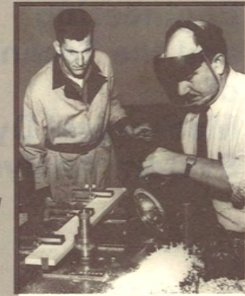
Stroboscopic photography revolutionized the study of motion and process. In this 1951 study, a researcher is using a strobe light to analyze the machining characteristics of woodcutting.
