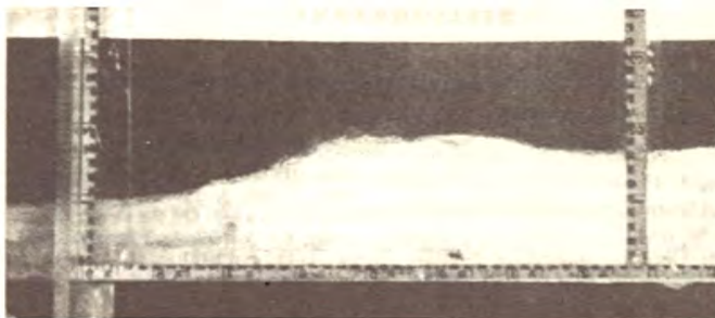
This photo shows the interfacial surge and almost horizontal free-surface between two fluids from Yih's work on hydraulic jump with C.R. Guha.
