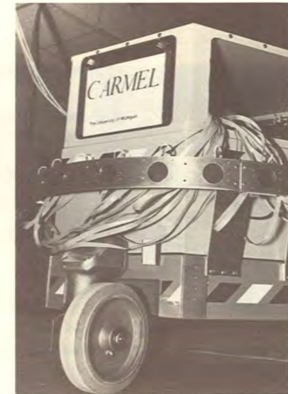
The obstacle-avoidance system of the CARMEL robot developed by MEAM researchers allows for high-speed obstacle avoidance. (see page 69 for more on CARMEL).
