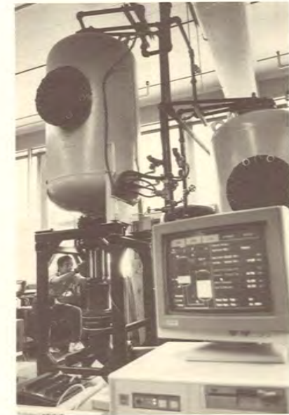
The fluid mechanics of cavitation is investigated in Prof. Steven Ceccio's laboratory. Cavitation is an important phenomenon because it adversely affects the functioning of hydromachinery. This blow-down apparatus induces cavitation by generating intense short duration surges through a three-inch diameter test section.
