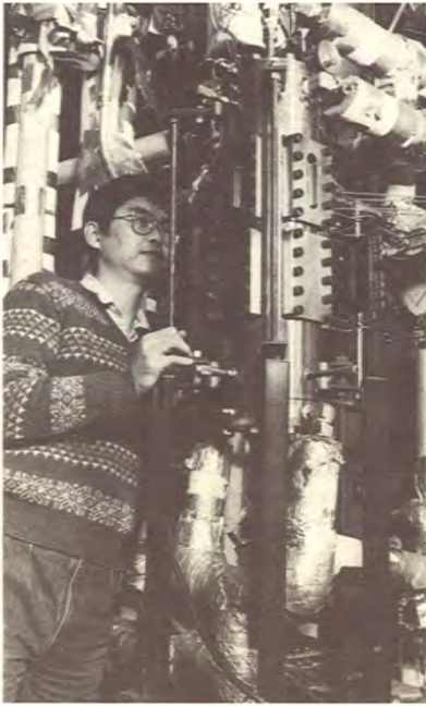
Investigations into the improvement of power engineering have been carried out in the Department of Mechanical Engineering and Applied Mechanics since 1868. This study by Prof. Herman Merte Jr. investigated boiling behavior at a plate/tube interface. This behavior is a regular source of stress fracture of tubing inside nuclear steam generator vessels.
