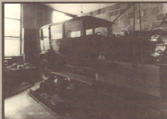
This early version of a chassis dynamometer permitted operation of a complete automobile at various loads and speeds. The experiment shown was an investigation of automobile noises produced during operation.
