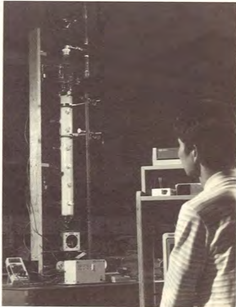
Steam injection into a packed column of glass particles, steam condensation, and the propagation of this condensation front are observed using this experimental apparatus in Prof. Massoud Kaviany's laboratory. This is part of a study concerning decontamination of soils using steam injection.
