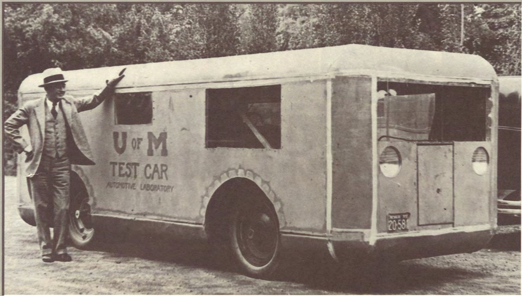
Mounted on a Chevrolet chassis, the "Blue Bird" served as one of the university's first test vehicles. Its exotic design helped to determine air resistance to motion in land vehicles, and to explore the effect of changes in vehicle shape. In the days before strain gauges, Lay suspended the shell of the "Blue Bird" on an assembly of scales to measure wind resistance while driving.
